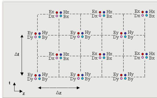
Figure 1. Modified FDTD mesh for bi-isotropic media.
