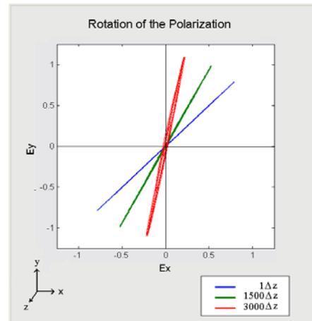
Figure 3. Polarization of the electric field at  $1\Delta z$ ,  $1500\Delta z$  and  $3000\Delta z$  from the source. The polarization rotates clockwise as the wave propagates in the medium
