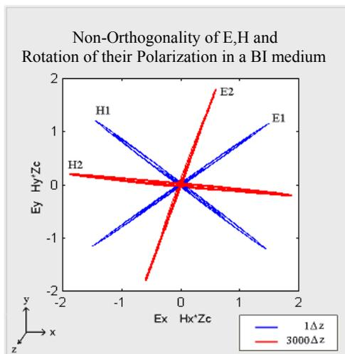
Figure 6. Rotation of the polarization and non-orthogonality of E and H at the points  $1\Delta z$ , and  $3000\Delta z$  from the source. The polarization is rotated clockwise (looking in the direction of propagation) as the wave propagates in positive  $z$ -direction. The Tellegen parameter fixes the angle between E and H to 102 degrees
