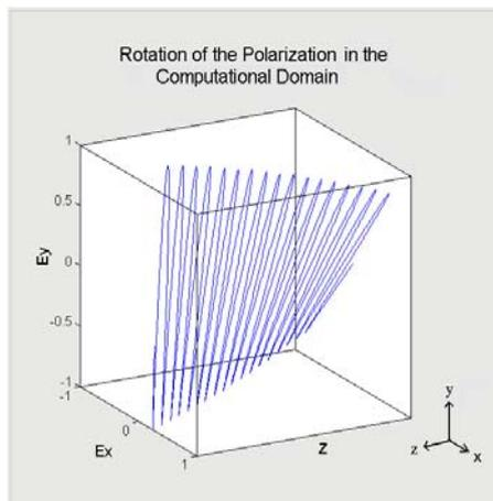
Figure 2. Rotation of the polarization of a wave propagating in a chiral medium. The figure shows the orientation of the electric field in part of the computational domain at time  $t=4000$  ps
