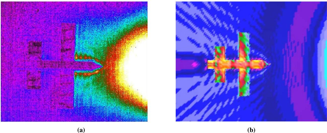
**Figure 4. Nose-On at 6GHz (Incident Spherical Wave)**
