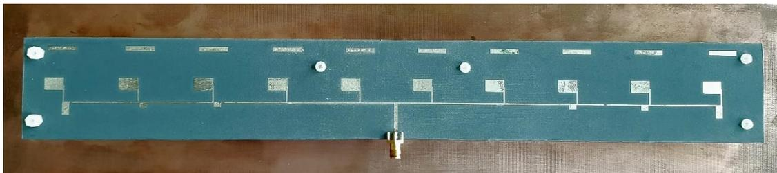
Fig. 10. Fabricated antenna array.
