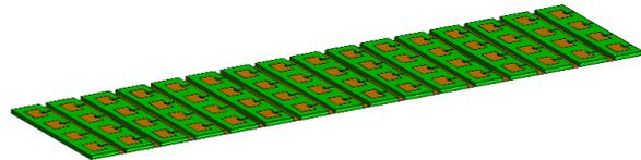
Fig. 2. The structure of antenna array composed of 64 microstrip patch antennas at the operating frequency of 14.5 GHz.
