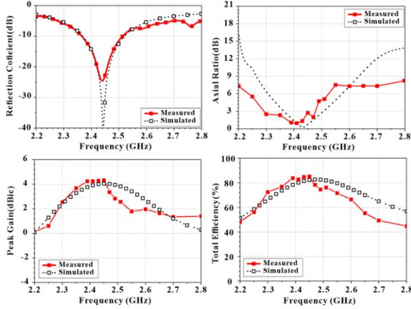
Fig. 4. Simulated and measured results of proposed antenna according to frequency: (a) reflection coefficients, (b) axial ratio, (c) peak gain, and (d) total efficiency
