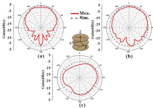
Fig. 5. Simulated and measured radiation patterns of the proposed antenna at 2.45GHz: (a)  $xy$ -plane, (b)  $yz$ -plane, and (c)  $xz$ -plane.
