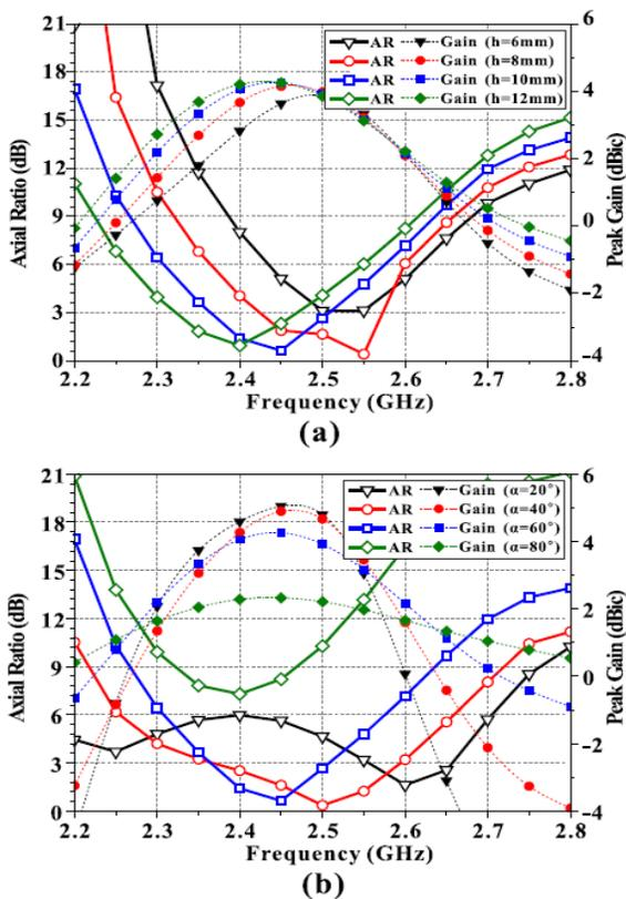
Fig. 2. Simulated axial ratio and peak gains of the proposed antenna with regard to the design parameters: (a) spacing distance,  $h$ , and (b) rotation angle,  $\alpha$ .
