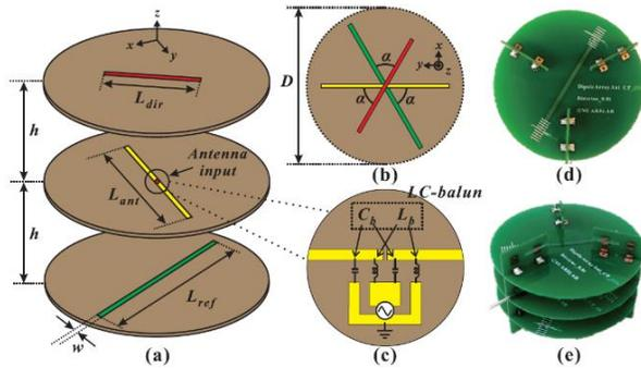
Fig. 1. Geometry of the proposed rotated stacked Yagi antenna configuration and its prototype: (a) perspective view, (b) top view, (c) expanded view of antenna input, (d) top view of fabricated antenna prototype, and (e) side view of fabricated antenna prototype.
