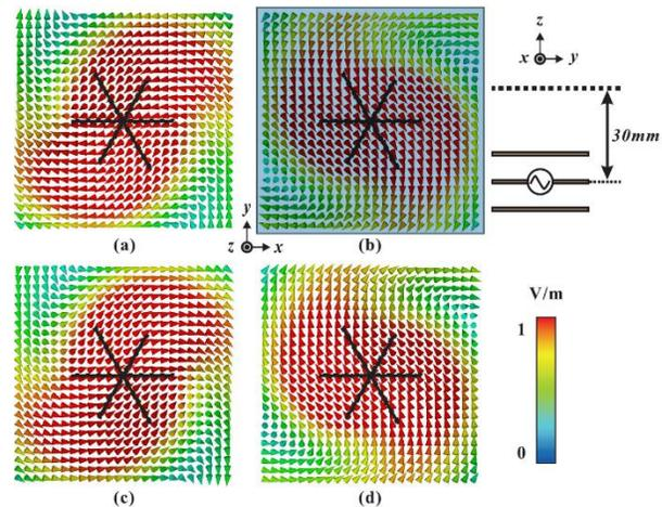
Fig. 3. E-field distributions at  $xy$  plane of 30mm away from the driven element in the proposed antenna with regard to the phase variation: (a) 0°, (b) 90°, (c) 180°, and (d) 270°
