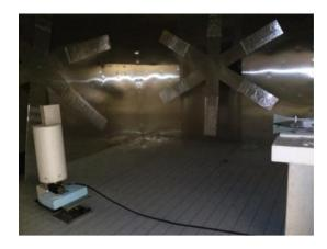
Fig. 2. Particular of the inner IUN RC with the flat S1 and S2 stirrers, the antennas in pseudo-monostatic configuration and with the dihedral corner reflector on the Microcontrole ITL 09 rotating table.
