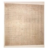
Fig. 22. The prototype of the dual-band Jerusalem-cross FSS with substrate. The geometrical parameters of the FSS are p = 7.577, w = 0.6059, s = 0.1294, h = 0.3793, d = 4.931, t = 0.035, and T = 0.8. Unit: mm.
