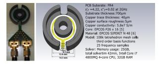
Fig. 5. Photo and model of the test loop antenna.
