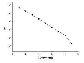
Fig. 3. HSS solution error in iterative refinement step.
