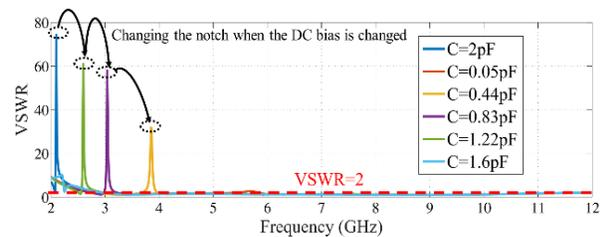
Fig. 4. VSWR of the slotted microstrip antenna.
