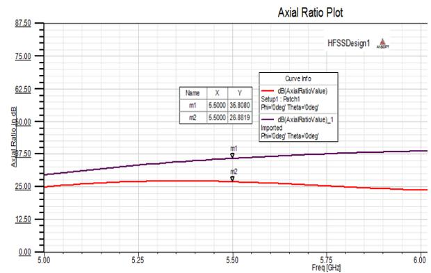
Fig. 6. Variation of axial ratio with frequency.
