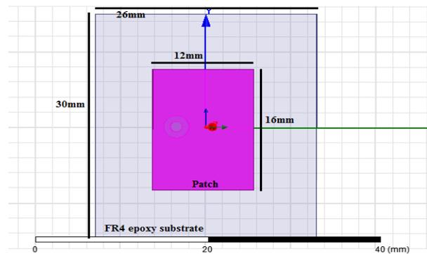
Fig. 1. Simulated top view of rectangular MPA.
