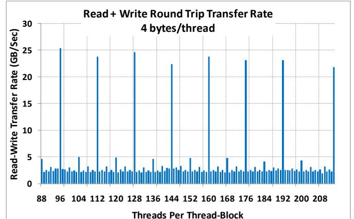
Fig. 5. GPU performance differences between coalesced and non-coalesced memory configurations.
