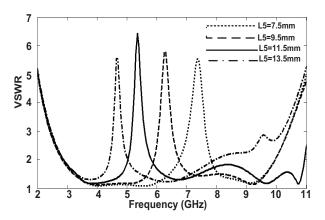
Fig. 6. Simulated VSWR characteristics of the antenna with a pair of L-shaped arms with different values of L5.
