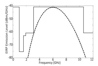
Fig. 13. Power spectrum density compared to FCC mask.
