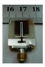
Fig. 9. Photograph of the realized antenna.
