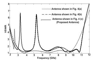
Fig. 5. Simulated VSWR characteristics for antennas shown in Fig. 4.
