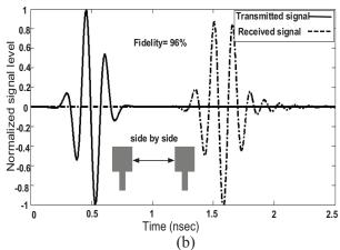
Fig. 14. Transmitted and received pulses in time domain for a UWB link with identical antennas without notches in: (a) face-to-face and (b) side by side orientations.
