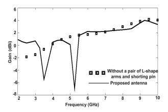
Fig. 11. Measured gain of the antenna without and with stop bands.
