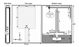
Fig. 1. Geometry of proposed antenna: Wsub=17, Lsub=21, Lp=12, Wp=10, Wf=1.9, Lf=8, Wg=8, Lg=4.5, d=1, L1=3, L2=13, L3=3.5, L4=1.5, L5=11.5, L6=1.25, L7=1.5, L8=1.5, L9=1, L10=5, S=0.5, h=1, and εr=4.4.
