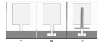
Fig. 2. (a) The ordinary square antenna, (b) the antenna with an inverted T-shape notch on the ground plane, and (c) the antenna with a pair of L-shaped arms on the back (DGS technique).
