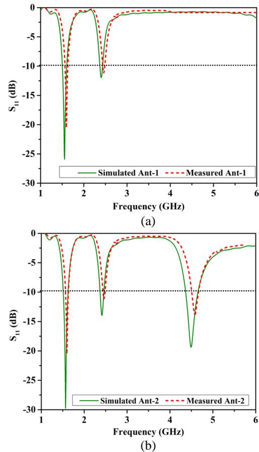
Fig. 3. S parameter: (a) Ant-1 and (b) Ant-2.
