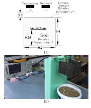
Fig. 8. Experimental setup of the ground penetrating radar with single receiver antenna: (a) schematic and (b) realized.
