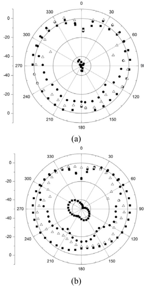
Fig. 5. Measured E-plane copolarization patterns (solid square: 2600MHz(both co- and X- pol); solid circle: 5800MHz; open uptriangle: 9300MHz). (a) Conventional monopole antenna, (b) proposed antenna.
