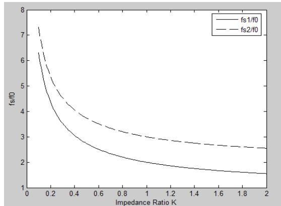
Fig. 3. High-order resonance frequency of the SIR.
