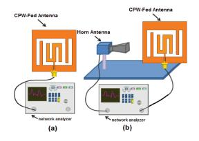
Fig. 9. Measurement set-up of the proposed antenna: (a) return loss, and (b) antenna gain and radiation patterns.
