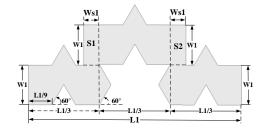
Fig. 4. Structure of quasi-second order Koch fractal element with  $W_{sl}=1.9 mm$ .
