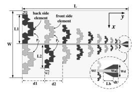
Fig. 1. Configuration of the proposed QLPK<sup>2</sup>DA.
