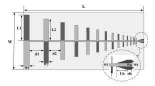
Fig. 2. Configuration of the LPDA.
