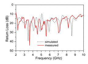
Fig. 9. Measured and simulated return loss of LPDA.
