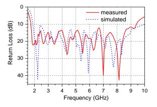
Fig. 20. Measured and simulated return loss of the conformal antenna.
