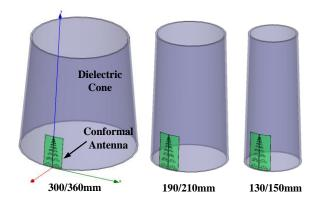
Fig. 14. Configuration of QLPK<sup>2</sup>DA mounted on cones with different curvatures.
