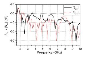
Fig. 22. Measured coupling of the conformal antenna.
