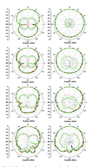
Fig. 16. Simulated radiation patterns of conformal antenna.  $-\blacksquare$  - co-polarization (300/360 mm), --- cross-polarization (300/360 mm),  $-\blacktriangle$  - co-polarization (190/210 mm), - - cross-polarization (190/210 mm), -• - co-polarization (130/150 mm), — cross-polarization (130/150 mm).
