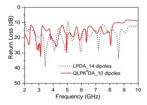
Fig. 5. Comparison of simulated return loss between LPDA and QLPK<sup>2</sup>DA.
