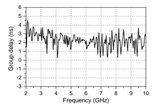
Fig. 13. Measured group delay of the proposed antenna.
