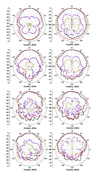
Fig. 11. Measured and simulated radiation patterns of QLPK<sup>2</sup>DA. -  $\blacktriangle$  - measured co-polarization, - $\bullet$ - measured cross-polarization, - $\nabla$ - simulated co-polarization, - $\circ$ - simulated cross-polarization.
