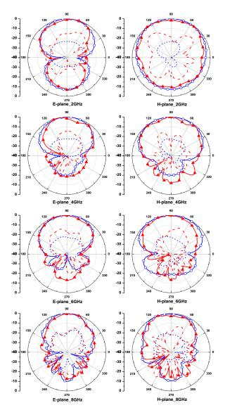
Fig. 21. Measured and simulated radiation patterns of conformal antenna. - $\circ$ - simulated co-polarization, --- simulated cross-polarization, - $\blacktriangle$ - measured co-polarization, --- measured cross-polarization.
