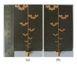
Fig. 8. Prototype of QLPK<sup>2</sup>DA: (a) front view and (b) back view.
