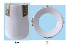
Fig. 19. Prototype of four QLPK<sup>2</sup>DA mounted on a dielectric cone: (a) side view and (b) top view.
