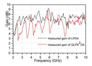
Fig. 12. Measured gain of LPDA and QLPK<sup>2</sup>DA.
