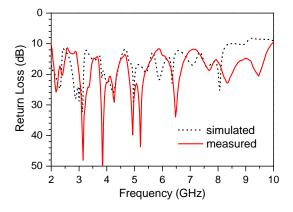
Fig. 10. Measured and simulated return loss of QLPK<sup>2</sup>DA.
