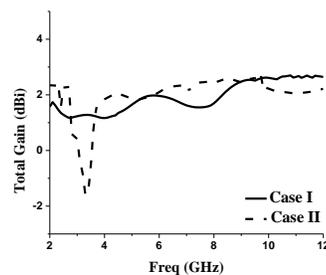
Fig. 9. Gain of proposed antenna.
