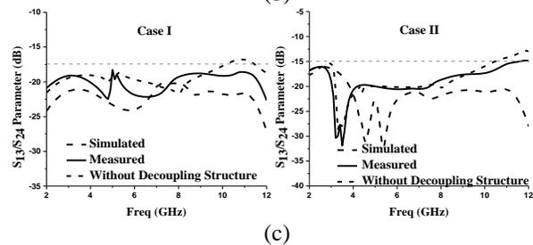
Fig. 7. Mutual Coupling with and without decoupling structure: (a) side-by-side, (b) diagonal, and (c) across.
