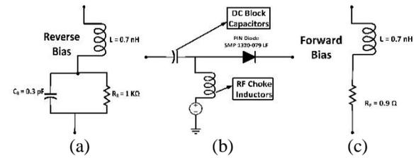
Fig. 2. Equivalent circuit model of PIN diode: (a) Case I, (b) biasing network, and (c) Case II.
