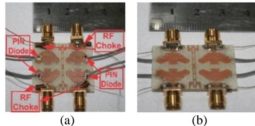
Fig. 3. Fabricated design: (a) front view and (b) back view.
