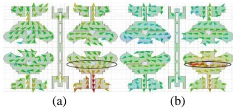
Fig. 4. Surface current density  $J_{surf}$  at 3.5 GHz: (a) Case I and (b) Case II.
