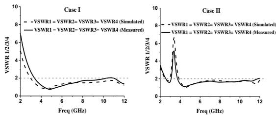
Fig. 5. Impedance matching of proposed prototype.
