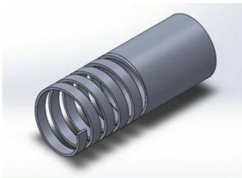
Fig. 12. Cylindrical conductor which is cut helically.
