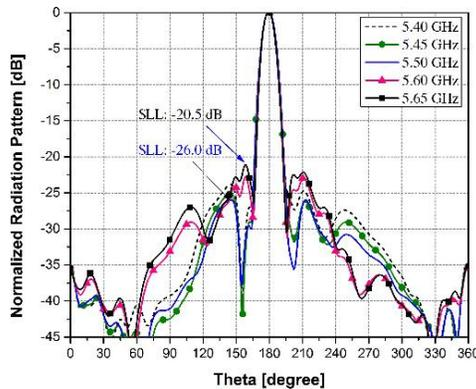
Fig. 12. The radiation pattern over different frequencies.
