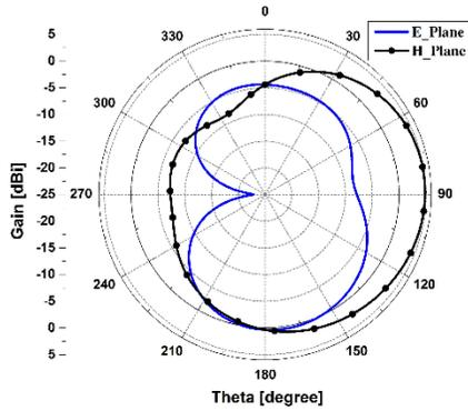
Fig. 3. Radiation pattern of the DSPD.
