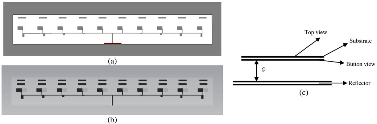
Fig. 9. Structure of the proposed array: (a) top view, (b) bottom view, and (c) side view.
