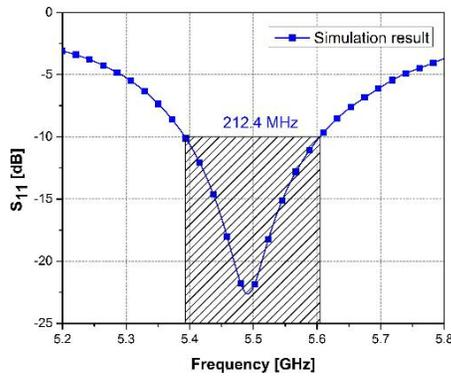
Fig. 11. Simulated  $S_{11}$  of the array [15].
