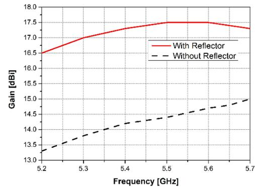
Fig. 14. Comparison of gain between the array with and without reflector.
