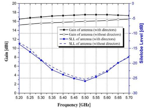
Fig. 13. The gain and SLL over the operating bandwidth.
