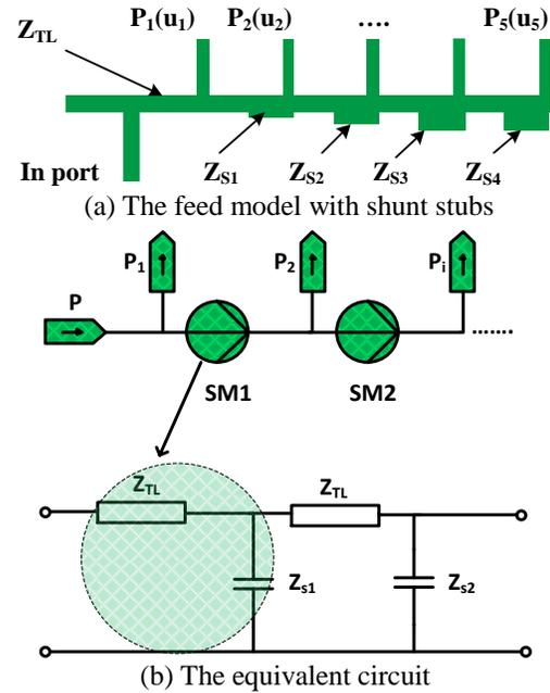
Fig. 5. The series fed network and its equivalent circuit.
