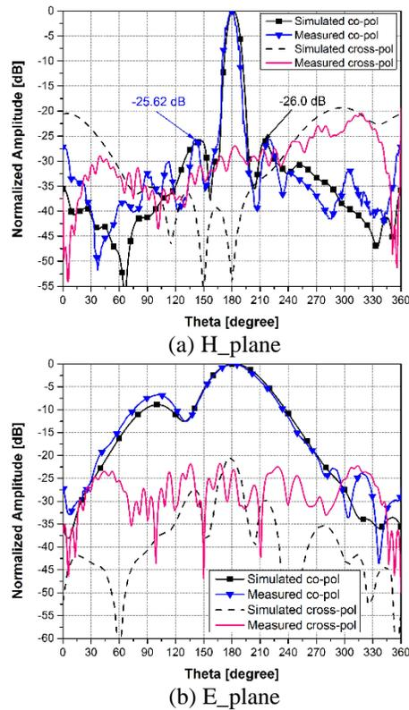
Fig. 16. Normalized radiation pattern of proposed array antenna at 5.5 GHz.
