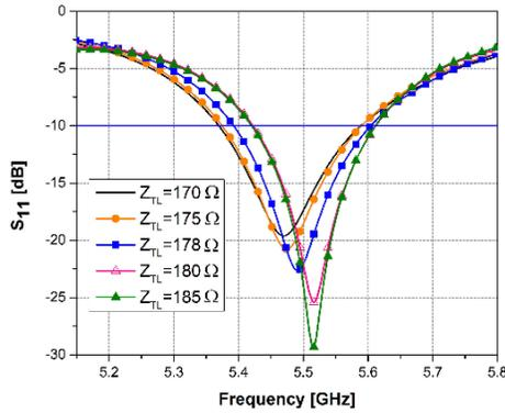
Fig. 6. The simulated reflection coefficient of different main line impedances.
