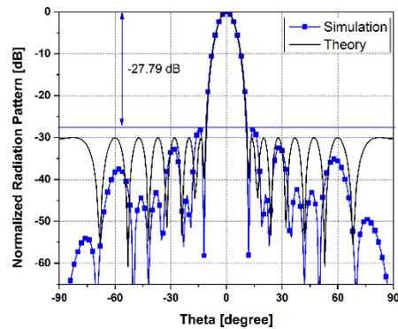
Fig. 8. Normalized radiation patterns with respect to the output power coefficient (solid line) and theoretical one (dotted line) [21].
