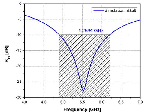
Fig. 2. Simulated  $S_{11}$  of the DSPD.
