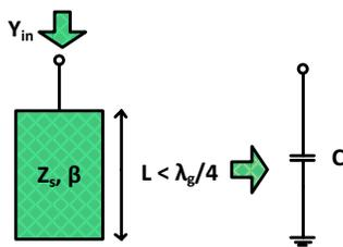
Fig. 4. The equivalent capacitor of shunt stub.
