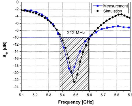
Fig. 15. The reflection coefficient of the array antenna.
