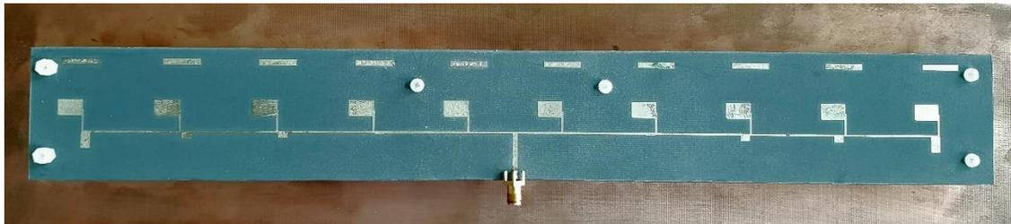
Fig. 10. Fabricated antenna array.
