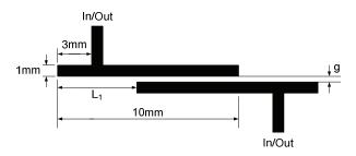
Fig. 3. Geometry of the second-order tapped-line microstrip filter [19].
