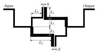
Fig. 8. Geometry of the  $2^{nd}$  -order CCDBR filter [19].
