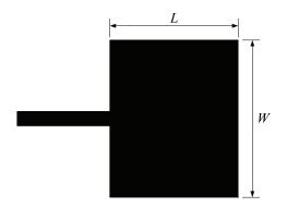
Fig. 6. Geometry of the patch antenna [21].
