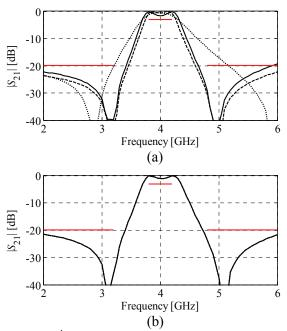
Fig. 9.  $2^{nd}$ -order CCDBR filter: (a) responses of  $R_f$  (solid line) and  $R_c$  (dashed line) at initial design  $x^{(0)}$  and response of  $R_f$  at  $x_c$  (dotted line); (b) response of  $R_f$  at the final design.
