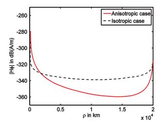
Fig. 3. The magnetic field  $|H_{\phi}|$  in A/m at f=100 Hz with a=6378 km,  $\phi = \pi/4$ ,  $\sigma_g = 10^{-5}$  S/m, h=85 km, and  $\beta = 0.3$  km<sup>-1</sup>.
