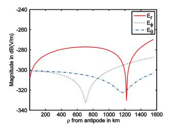
Fig. 4. Magnitudes of the components  $E_r, E_{\theta}, E_{\phi}$ at f=100 Hz with a=6378 km,  $\phi = \pi / 4$ ,  $\sigma_g = 10^{-5}$  S/m, h=85 km, and  $\beta =0.3$  km<sup>-1</sup>.
