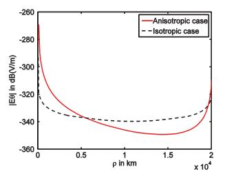
Fig. 2. The electric field  $|E_{\theta}|$  in V/m at f=100 Hz with a=6378 km,  $\phi = \pi / 4$ ,  $\sigma_g = 10^{-5}$  S/m, h=85 km, and  $\beta = 0.3$  km<sup>-1</sup>.
