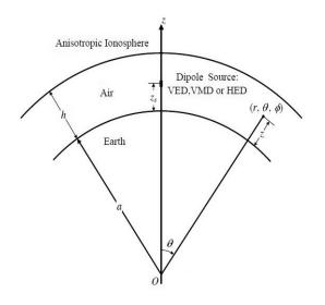
Fig. 1. Geometry of a dipole source in the presence of an anisotropic earth-ionosphere cavity.
