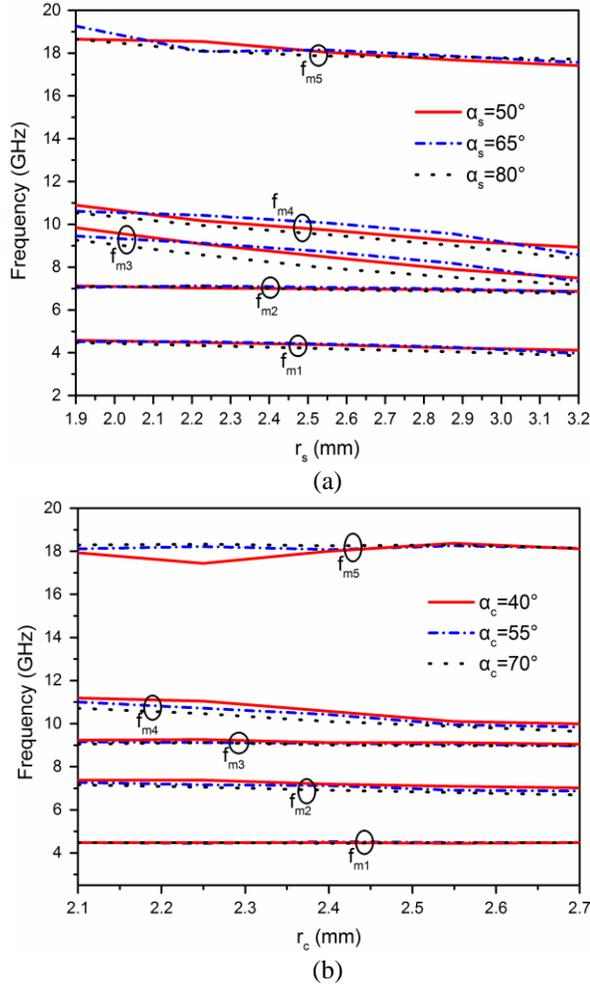
Fig. 3. Simulated characteristics of the proposed radial-stub loaded structure under weak coupling case with varied: (a)  $\alpha_s$  and  $r_s$ , (b)  $\alpha_c$  and  $r_c$ , where the other dimensions are fixed as  $l_1 = 9.5$  mm,  $l_2 = 0.5$  mm,  $l_3 = 2.2$  mm,  $s_1 = 0.1$  mm,  $w = w_1 = 1.1$  mm.
