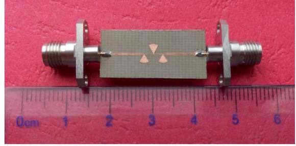
Fig. 4. Photograph of the fabricated microstrip UWB BPF.
