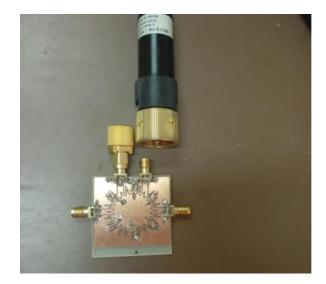
Fig. 3. A photograph of the measured coupler with bond wires and connectors (port 2 is match terminated).
