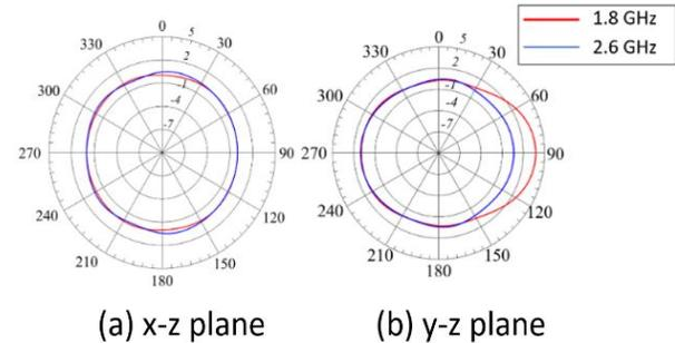
Fig. 6. Measured radiation patterns (gain in dBi) of the proposed antenna at 1.8 and 2.6 GHz: (a) x-z plane and (b) y-z plane.
