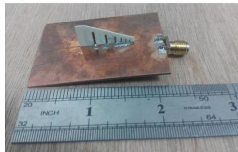
Fig. 6. Fabricated 6GHz-18GHz end-fire monopole log-periodic antenna
