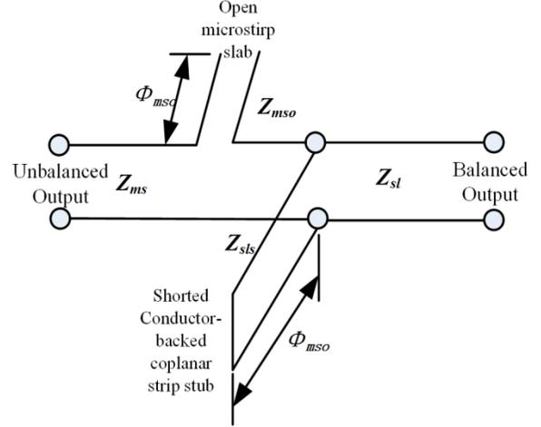
Fig. 2. Equivalent circuit of microstrip-to-slotline transition.
