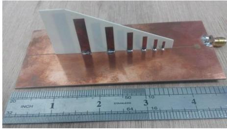
Fig. 3. Fabricated 2GHz-6GHz end-fire monopole log-periodic antenna
