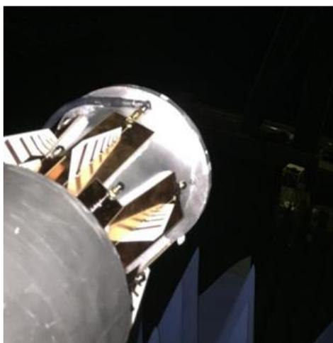
Fig. 10. 2 GHz-18 GHz monopole antenna array test picture.
