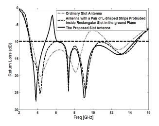
Fig. 3. Simulated return loss characteristics for the various structures of the antenna shown in Fig. 2.
