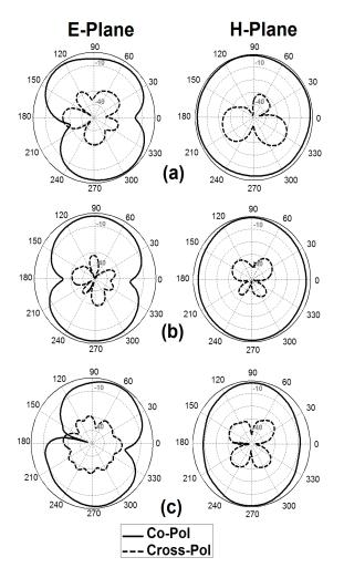
Fig. 8. Measured radiation patterns of the proposed antenna (a) 4 GHz, (b) 7 GHz, and (c) 10 GHz.
