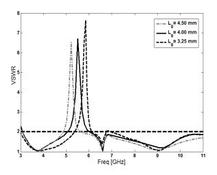
Fig. 5. Simulated VSWR for the proposed antenna with different values of  $L_{p}$ .
