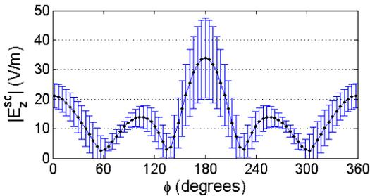
Fig. 6. Magnitude of the scattered electric field on a circle of radius 3.4 m. Error bars represent  $\pm 3\sigma$  deviation from the mean.
