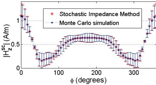
Fig. 2. Mean value of the magnitude of the scattered magnetic field. Error bars represent  $\pm 3\sigma$  deviation from the mean.
