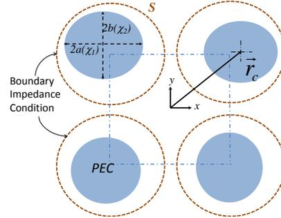
Fig. 3. Array of four PEC elliptical cylinders with random axes lengths and random positions.
