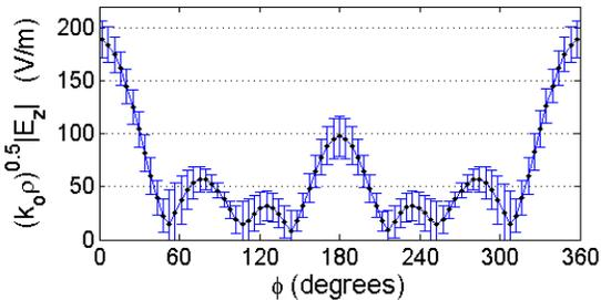
Fig. 7. Mean value of the magnitude of the far electric field at  $\rho = 1000/k_0$ . Error bars represent  $\pm 3\sigma$  deviation from the mean.
