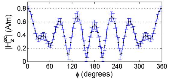
Fig. 4. Mean value of the magnitude of the scattered magnetic field on a circle of radius 3.8 m enclosing the four cylinders. Error bars represent  $\pm 3\sigma$  deviation from the mean.
