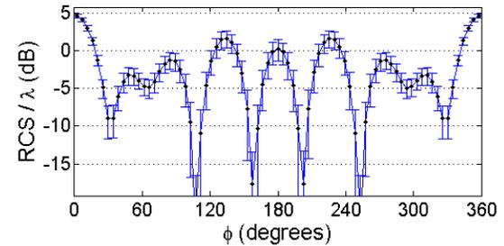
Fig. 5. Mean value of the radiation cross section (RCS) of the magnetic field. Error bars represent  $\pm 3\sigma$  deviation from the mean.
