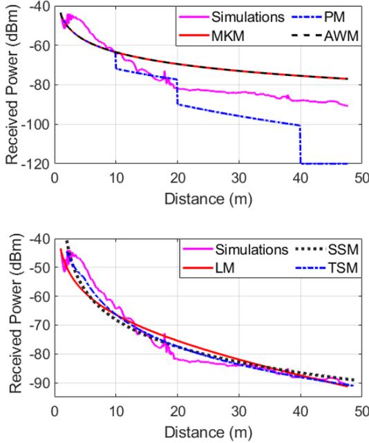
Fig. 6. RSS through the corridor at 28 GHz.
