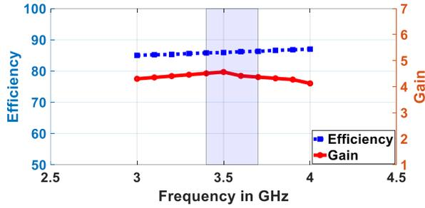
Fig. 13. Antenna gain and efficiency when the diode D<sub>1</sub> is ON and diode D<sub>2</sub> is OFF.
