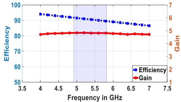
Fig. 17. Antenna gain and efficiency when the diodes D<sub>1</sub> and D<sub>2</sub>=ON.
