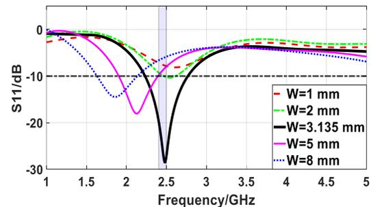
Fig. 3.  $S_{11}$  variation with frequency for various slot widths  $W$ , at  $L=34.55$  mm.
