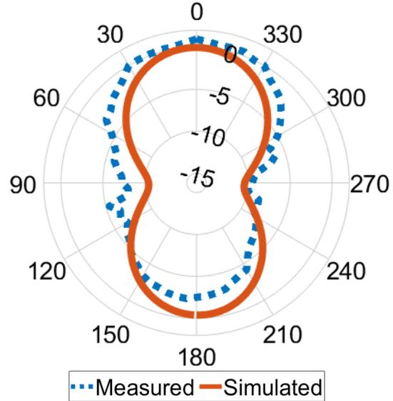
Fig. 16. Normalized simulated and measured radiation patterns of the antenna at 5.3 GHz and both diodes are in the ON state.
