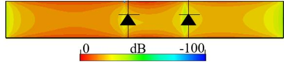
Fig. 15. Simulated E-field distribution in the slot (zooming on the slot), the diodes D<sub>1</sub> and D<sub>2</sub> are ON.
