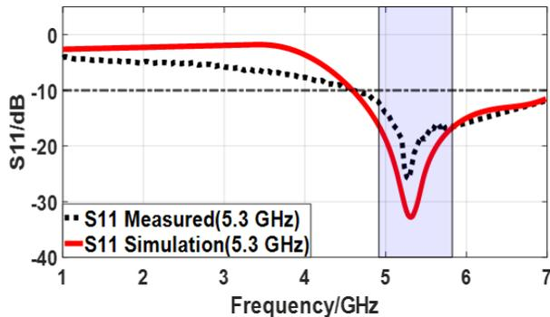
Fig. 14. Simulated and measured S<sub>11</sub> variation with frequency when both diodes D<sub>1</sub> and D<sub>2</sub> are in ON state.
