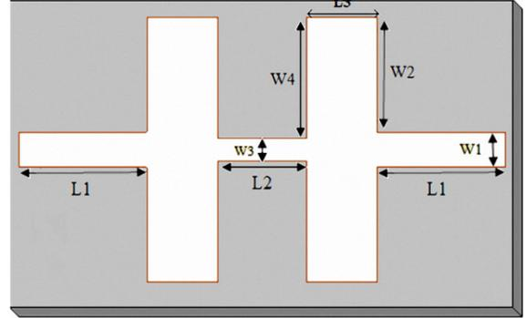
Fig. 8. Schematic of primary LPF.
