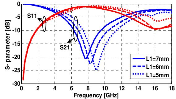
Fig. 6. Simulated S-parameter of H-type DGS for  $L1$  variation.
