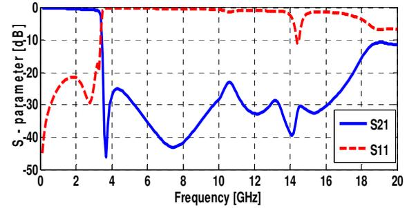
Fig. 11. Simulated frequency response of designed LPF.
