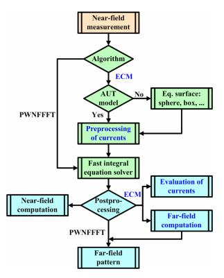
Fig. 4. Flowchart of near-field transformation.
