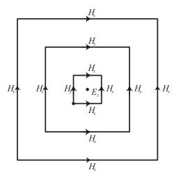
Fig. 1. *E* field multi-region decomposition for C-RK-HO-FDTD method.
