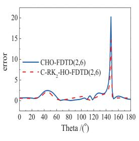
Fig. 8. Errors of the CHO-FDTD (2, 6) and C-RK<sub>2</sub>-HO-FDTD (2, 6) methods.
