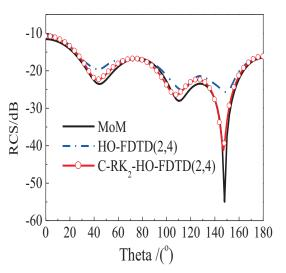
Fig. 5. RCS of *E*-plane bistatic in the dielectric cylinder of different methods.
