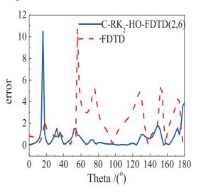
Fig. 13. Errors of the FDTD and C-RK2-HO-FDTD (2, 6) methods.
