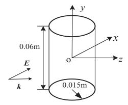
Fig. 4. Geometric model of the dielectric cylinder.
