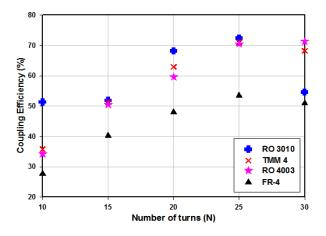
Fig. 3. Coupling efficiency of Witricity device with different substrates and varied number of spiral coil turns between 10 and 30.
