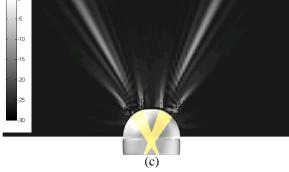
Fig. 2. Hybrid electromagnetic modeling of THz probe antennas: (a) discretization of the antenna slots with biquadratic mesh, (b) ray-tracing/physical optics analysis for the THz antenna radiation pattern in the presence of the hemispherical lens, and (c) computed *E*-field intensity distribution of both receiving and transmitting THz probe antennas.
