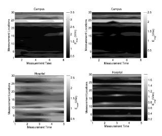
Fig. 2.  $E_{max}$ ,  $E_{avg}$  values versus location for campus and hospital.
