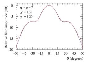
Fig. 5. E-plane pattern. Solid line: reconstructed from cylindrical NF data. Dashes: reconstructed from the NF data acquired along a spiral.
