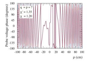
Fig. 4. Phase of  $V_{\varphi}$  on the radial line at  $\varphi = 0^{\circ}$ . Solid line: measured. Dashes: reconstructed from the NF data acquired along a spiral.
