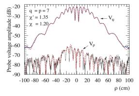
Fig. 2. Amplitudes of  $V_{\varphi}$  and  $V_{\rho}$  on the radial line at  $\varphi = 0^{\circ}$ . Solid line: measured. Dashes: reconstructed from the NF data acquired along a spiral.
