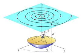
Fig. 1. Planar spiral scanning.
