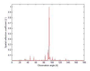
Fig. 12. Plot of spatial reflection coefficient as a function of bistatic RCS formulated with 90° signal incidence in satellite-to-aircraft scenario.
