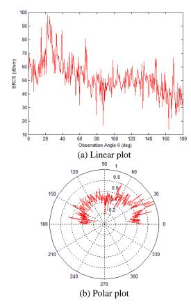
Fig. 8. RCS observation of signal incidence at  $\beta_{\rm B} = 158.079^{\circ}$  in satellite-to-aircraft communication scenario.
