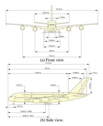
Fig. 4. Aircraft A380 detailed dimensions [27].
