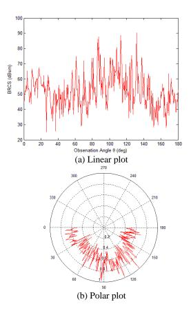
Fig. 9. RCS observation of signal incidence at  $\alpha_{\rm C} = 90^{\circ}$  in ground-to-aircraft communication scenario.
