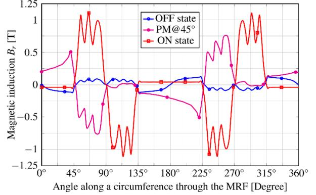
Fig. 5. The radial component of  $B$  along a circumference inside the MRF.
