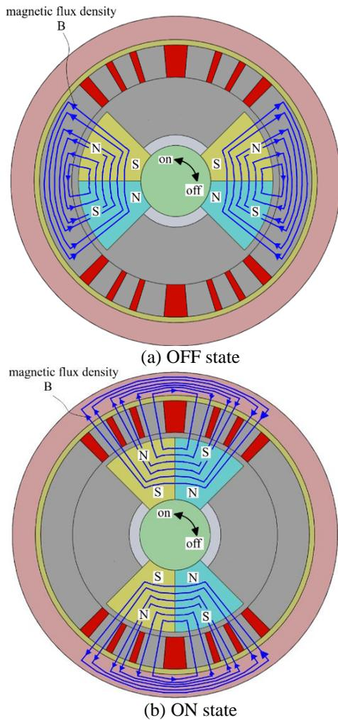
Fig. 2. The operation principle of the proposed brake.
