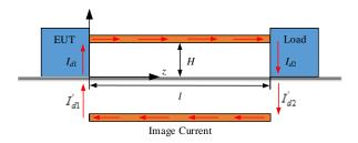
Fig. 6. A multi-dipole radiated model for cable-enclosure system.
