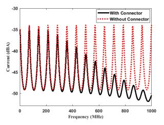
Fig. 10. A comparison of current distribution of load end with and without connectors.
