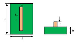
Fig. 7. The geometry and dimensions of PCB.
