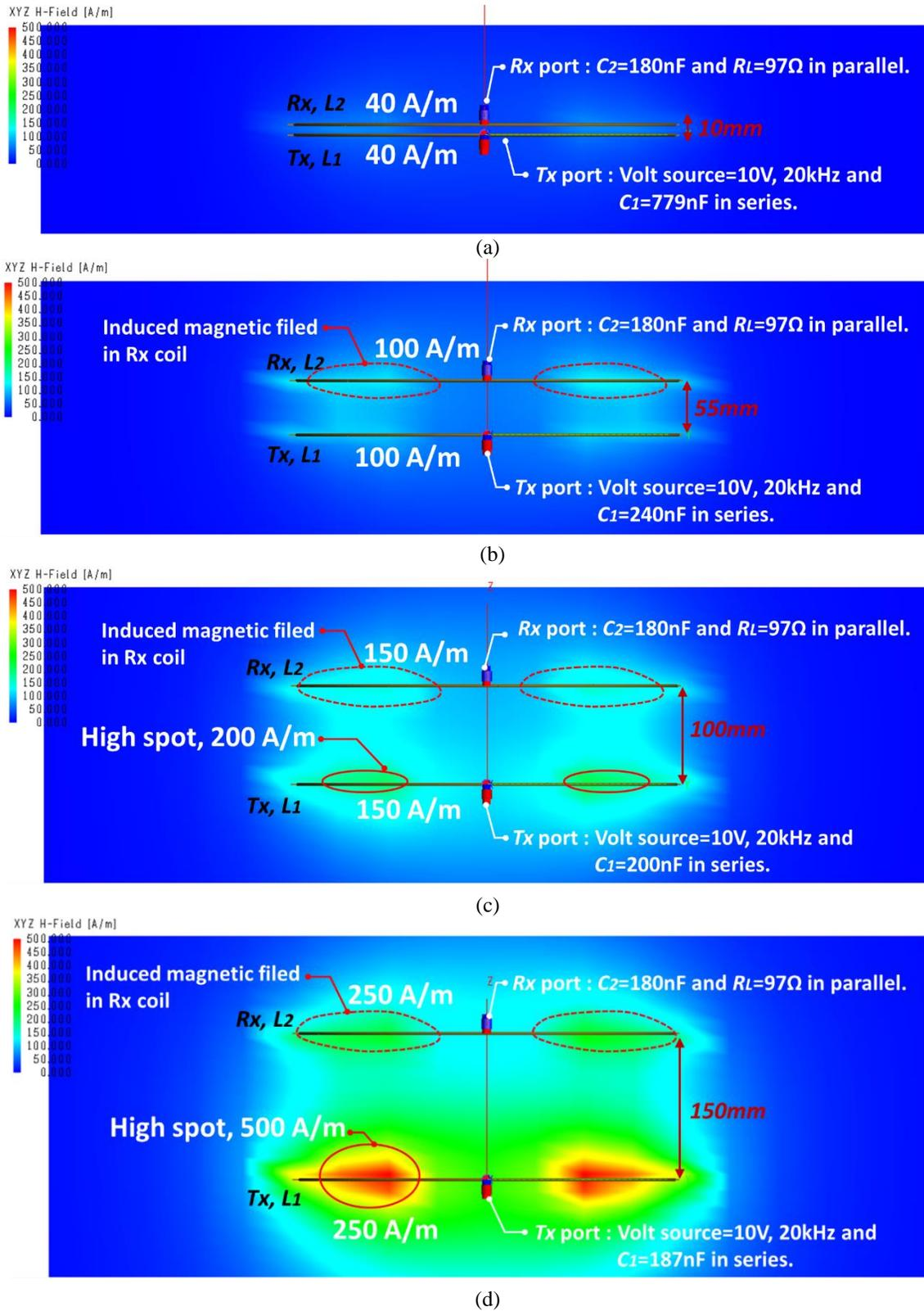
Fig. 7. Magnetic coupling and field distribution in SP topology over the different airgap ( $C_2 = 180\text{ nF}$ ) at 20 kHz: (a) 10 mm,  $C_1 = 779\text{ nF}$ , (b) 55mm,  $C_1 = 240\text{ nF}$ , (c) 100 mm,  $C_1 = 200\text{ nF}$ , and (d) 150 mm,  $C_1 = 187\text{ nF}$ .
