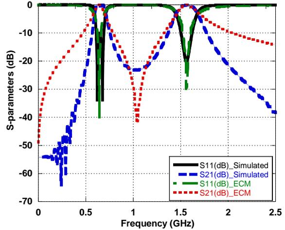
Fig. 3. Comparison between the equivalent circuit (ADS) and EM simulation (CST).
