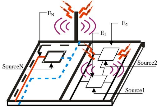
Fig. 1. Radiated EMI noise source model.
