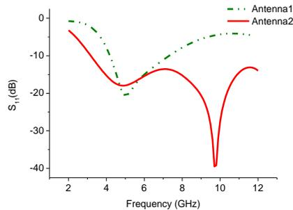
Fig. 2. Simulated  $S_{11}$  of antenna 1 and 2.
