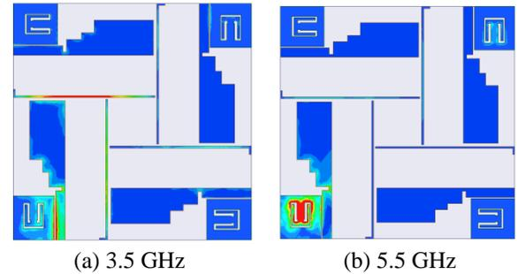
Fig. 12. Surface current distributions at (a) 3.5 GHz and (b) 5.5 GHz.
