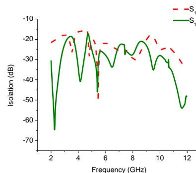
Fig. 5. Simulated isolation of the MIMO antenna.
