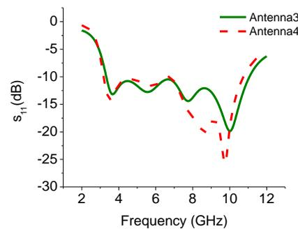
Fig. 4. Simulated  $S_{11}$  of antenna 3 and 4.
