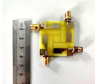
Fig. 9. Photograph of the fabricated MIMO antenna.
