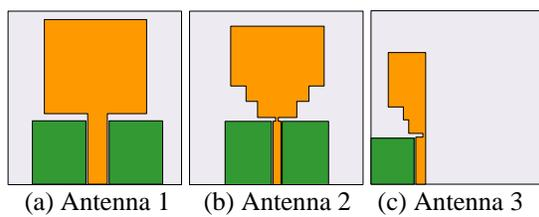
Fig. 1. Design of UWB MIMO antenna element.
