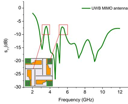
Fig. 8. Simulated  $S_{11}$  of proposed MIMO antenna.
