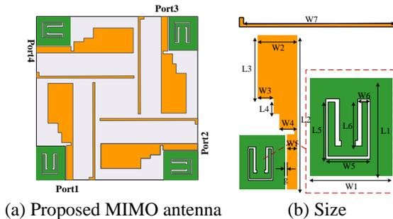
Fig. 7. Four-element UWB MIMO antenna with dual-notched.
