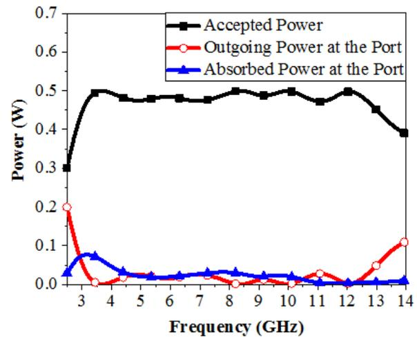
Fig. 6. Powers at the input of the antenna.
