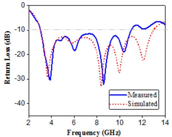
Fig. 9. Measured and simulated reflection coefficient of the proposed UWB CPW cauliflower-shaped antenna.
