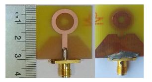
Fig. 10. Photograph of the fabricated antenna.
