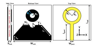
Fig. 1. Geometry of the proposed antenna.
