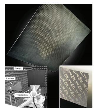
Fig. 6. The fabricated sample of design metasurface and its measurement system.
