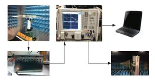
Fig. 5. Data acquisition setup for the AOA estimation experiment.
