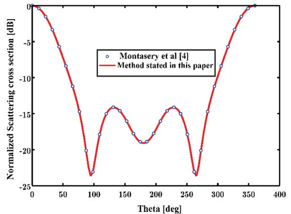
Fig. 6. Normalized co-polarization scattering cross-section with parameters  $\epsilon_1 = \epsilon_2 = \epsilon_3 = 9.8$ ,  $\mu_1 = 1$ ,  $\mu_2 = 19$ ,  $\mu_3 = 6$ ,  $\phi_0 = \pi/2$ ,  $M\eta_0 = \pm 1$ ,  $a = \lambda/6$ ,  $b = \lambda/3$ .
