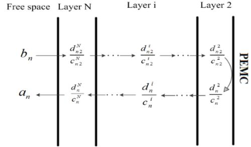
Fig. 2. Movements in layers in order to find scattering coefficient. Layers are cylindrical.
