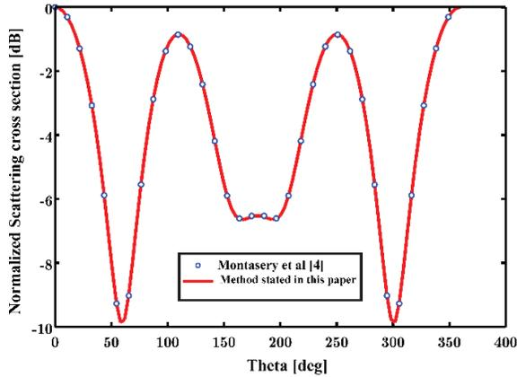
Fig. 7. Normalized cross-polarization scattering cross-section with parameters  $\epsilon_1 = 9.8$ ,  $\epsilon_2 = 16$ ,  $\epsilon_3 = 7$ ,  $\mu_1 = 1$ ,  $\mu_2 = 19$ ,  $\mu_3 = 6$ ,  $\varphi_0 = \pi/2$ ,  $M\eta_0 = \pm 1$ ,  $a = \lambda/6$ ,  $b = \lambda/3$ .
