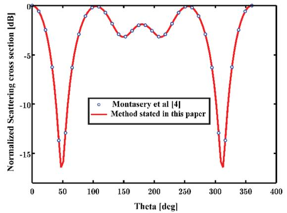
Fig. 5. Normalized cross-polarization scattering cross section with parameters  $\epsilon_1 = \epsilon_2 = \epsilon_3 = 9.8$ ,  $\mu_1 = \mu_2 = \mu_3 = 1$ ,  $\phi_0 = \pi/2$ ,  $M\eta_0 = \pm 1$ ,  $a = \lambda/6$ ,  $b = \lambda/3$ .
