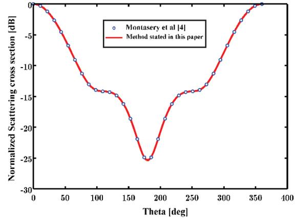
Fig. 4. Normalized co-polarization scattering cross section with parameters  $\epsilon_1 = \epsilon_2 = \epsilon_3 = 9.8$ ,  $\mu_1 = \mu_2 = \mu_3 = 1$ ,  $\phi_0 = \pi/2$ ,  $M\eta_0 = \pm 1$ ,  $a = \lambda/6$ ,  $b = \lambda/3$ .
