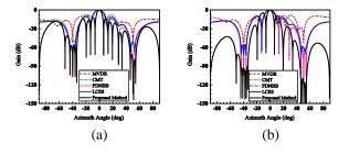
Fig. 2. (a) Normalized beampatterns of different algorithms when parameter  $\varepsilon$  is equal to  $6 \times 10^{-6}$ , and (b) normalized beampatterns of different algorithms when parameter  $\varepsilon$  is equal to  $6 \times 10^{-10}$ .
