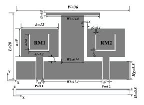
Fig. 1. The geometry of the proposed UWB MIMO antenna.
