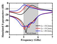
Fig. 4. Simulated  $S_{11}$  and  $S_{12}$  results of the proposed UWB MIMO antenna for different *Ls*.
