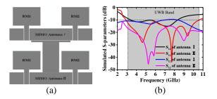
Fig. 2. Geometry (a) and simulated *S*-parameter (b) of the MIMO antenna I and MIMO antenna II.
